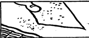
When sandpapering, place dampened newspaper under and around the object. This will catch and settle most of the dust.
