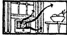
Wall panel heaters, with heating units behind decorative grilles, provide radiant heat with natural or fan-forced convection.
