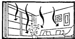
Ceiling cable is invisible. Wires less than 1/4" thick are concealed within ceilings. Each room's temperature is individually controlled.
