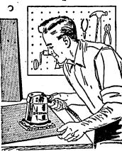
Three different grades of abrasive are enough to get a good finish on most material.
