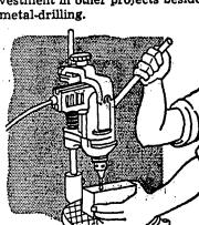
achieved by acquiring a stand that converts portable electric drill into drill press.
