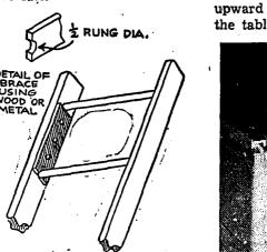
Ladder rungs can be reinforced with wood or metal.
