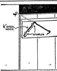
An angle hook for your barn door is easily made by bending a piece of 1/4-in, rod as indicated. Hook is pivoted inside the door by means of two large staples.
