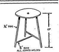
An old cultivator disc mounted on legs of 1/2-in, pipe makes a utility stool that is quite handy around the farm or in the shop. Legs are welded to the convex side of the disk and are brared with two lengths 38-in. rod, as shown.
