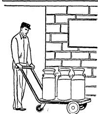
Three-wheeled cart saves labor in handling milk cans around the dairy barn. Low bed eases the labor of lifting cans and single rear wheel permits making sharp turns.
