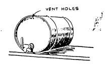
One of the simplest ways of venting an outdoor drum which is mounted horizontally is to drill two ventholes just under the rim. Fuel will then flow freely and overhang of rim will prevent moisture from entering through the holes.
