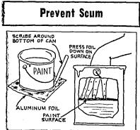
to a paint job and find that paint scum has formed. Scum will not form in a closed can if you cover the paint surface with a disc of aluminum foil before storing it away. Set can over aluminum foil and scribe around it to cut disc to proper size. Push foil disc into can and down to paint level. Later, simply pinch and lift off foil, stir paint and begin
