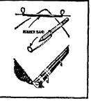
One sure way for those school youngsters of yours to keep a pencil at hand inside the cover of a notebook is to insert a rubber band through two holes punched in the cover. Notice in the drawing that the band is knotted near each end to provide loops for the pencil and also to keep the band in place. A small ruler, dividers and other school equipment can be carried in the same way. A flat rubber band is preferable to a round one for this particular purpose.
