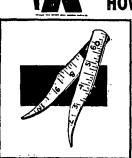
A folding rule, once broken, is generally considered useless and simply thrown out of the home workshop. However, here is a handy comparative caliper, useful for taking both inside and outside rough measurements, made from just such a broken folding rule. Two 6-in. sections are easily cut to the shape shown in the sketch by cutting on a jigsaw or by filing. Fine sandpaper can be used to smooth off any remaining rough edges.
