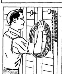
Handy wall hangers for the garage or barn can be had by using discarded auto valves. Because their heads are large in comparison with the stems, such hangers will support all types of miscellaneous gear. Make holes slightly smaller than valve stems, drill at an angle, then drive valves into the wall at least one third the length of the
