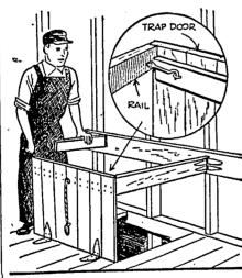
If you have a trap door in your barn loft, here is an idea that could possibly save you a dangerous fall. Fit it with guardrails as shown above. The rails, which are hinged to the barn wall, swing outward and are hooked to the trap door when it is in the upright position. When the door is closed the rails are folded flush against the wall.
