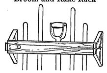
The life of brooms, hoes, rakes or pitchforks used around the barn will be materially increased if rack is made so that they may be hung on the wall. This rack needs only scrap lumber and a hinge. If necessary a leather hinge may be used.
