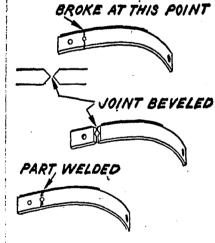
The operator of the farm machinery repair shop can repair a broken bumper or similar part. In this case it was broken at the point shown in the sketch. The joint was beveled in the manner shown and welded with 1/8-inch fleetweld 37", using 120 amperes.
