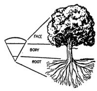
Face, body and root are important in electric welding. Drawingcourtesy Lincoln Electric Co.
